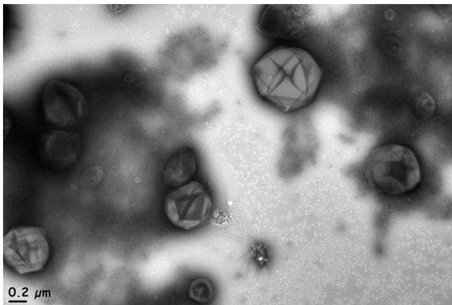
Figure S13 | TEM image of spheres found initially after mixing (\text{Nce-Npe})_{18} and (\text{Nae-Npe})_{18} . Immediately after the mixing, 20 \mu\text{L} of the solution was dropped on a carbon coated copper grid and incubated for ten minutes to ensure the adsorption of peptoids. The grid was incubated with a droplet of negative staining solution (Nano W ® , Nanoprobes Inc., Yaphank, NY) for two minutes and then with a droplet of water for two minutes. We repeated the staining procedure once and soaked up the remaining solution on the grid with filter paper.
