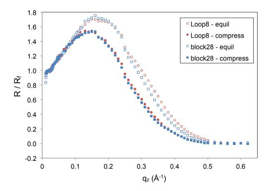
**Figure S3**. Fresnel-normalized reflectivity data obtained from the Peptoid **1** (blue) and **3** (red) monolayers at equilibrium surface pressure (open symbols) and after compressing each peptoid monolayer to a fixed surface pressure of 37 mN/m (closed symbols). Error bar (vertical line), corresponding to the standard deviation, is included with each point.
