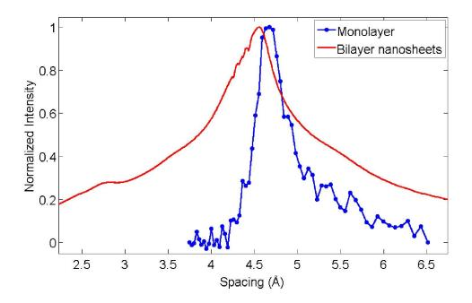
**Figure S2**. Comparison of the grazing incidence X-ray diffraction peak obtained from the Peptoid **3** monolayer at the air-water interface, after compressing the monolayer to a fixed surface pressure of 37 mN/m (blue), and the powder X-ray diffraction peak obtain from a dry pellet of Peptoid **3** nanosheets (red), at the 4.6 Å spacing, corresponding to the lateral distance between neighboring polymer chains.
